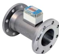
Made possible with hybrid technology which combines two sensors of different principles, vortex and thermal, the Hybrid Multi DELTA is capable of measuring extra-wide flow ranges as wide as 1:900 with just one unit. This flowmeter is optimal for managing the usage of compressed air.
