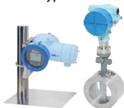
The DELTAFLOW Type F measures the flow rate by detecting the vortices generated by flow velocity change in the following manner; temperature change in thermistor sensor → resistance change → pulses proportional to the flow velocity.
