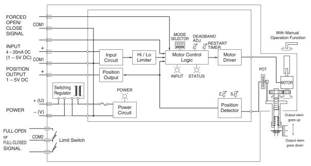
Full-open/-closed signals and forced open/close signals are optional. Disregard the switching regulator circuit for DC power input.
