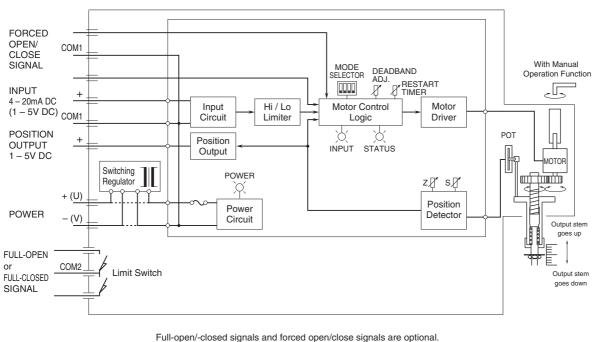
Disregard the switching regulator circuit for DC power input.
