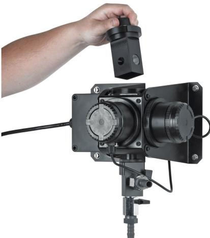
Figure 5 Dry standard calibration
