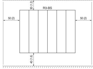
Panel bottom or wiring conduit (height ≤ 50 mm or 2 in.)
