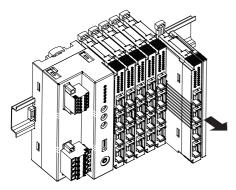
Removing an intermediate module
