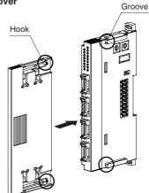
The protective cover is to be attached over the connected  $\ensuremath{\mathsf{I/O}}$  module at the right end.
