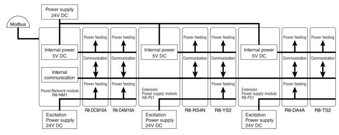
Note 1: Use same power source for Power/Network module and Extension power supply module. Note 2: Extension power supply module can be used up to two units at the same time.
