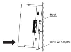
Position the upper hook at the rear on the DIN rail and push in the lower. When removing the module, push down the DIN rail adaptor utilizing a minus screwdriver and pull.
