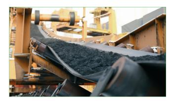
The application LaseBVC - Bulk Volume Conveyor is a highly precise two-dimensional measurement system especially developed for the measurement of materials on conveyor belt systems.
