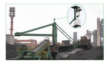
The application LaseBVH - Bulk Volume Measurement is a highly precise three-dimensional measurement system especially developed for measurements in heaps or piles.
