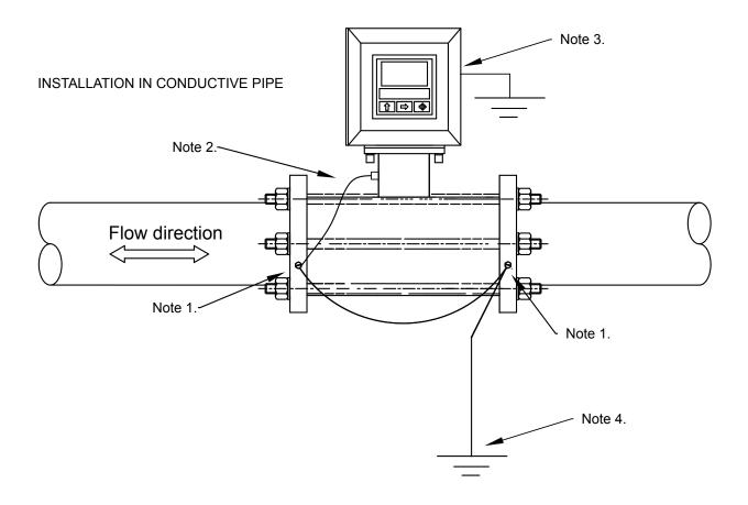
Note 1. Using a #21 (0.159") drill bit, drill a ½" deep hole in edge of each mating flange. Tap each hole using a 10-32 tap. Secure the ring connectors (provided) and grounding wires to the flange using the green grounding screws (provided).
