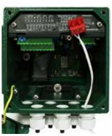
**Step 4** Remove electrode and coil connectors from their sockets.
