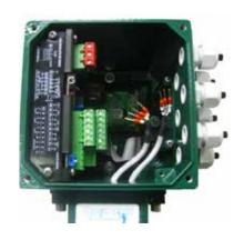
Step 6 Remove mounting screws from the bottom of the enclosure. Screws do not need to be fully removed.
