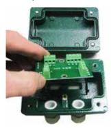
Step 2 Feed the cables through the holes in the bottom of the junction box and mount it in place.
