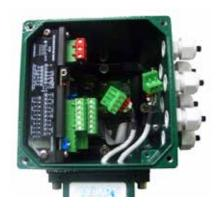
**Step 5**Remove electrode and coil wires from connectors and set aside.
