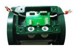
Step 4 Attach the cables to the terminal blocks as shown.
