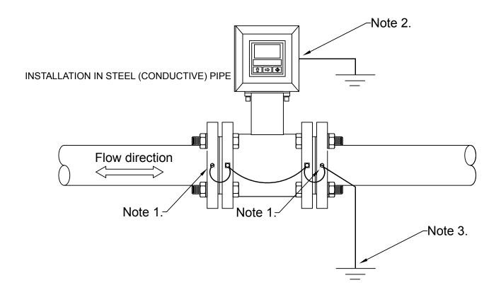
Note 1. Using a #21 (0.159") drill bit, drill a ½" deep hole in edge of each mating flange. Tap each hole using a 10-32 tap. Secure the ring connectors (provided) and grounding wires to the flange using the green grounding screws (provided).
