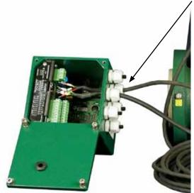
Connect the coil and electrode wires to the appropriate terminals according to the numbered tags on each wire.
