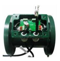
Step 6 Cables should be connected as shown.
