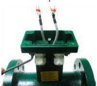
Step 3 Re-install the circuit board.
