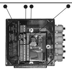
Opto-coupled open collector pulse outputs
