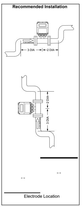
Place pipe at least 3 pipe diameters downstream and 2 pipe diameters upstream from bends and obstructions.
