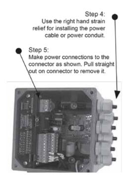
Step 6: Wire the connector as shown based on input power requirements of the transmitter. Earth connection must be made.
